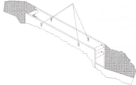
6. **WARNING:** Lift eyes are designed and intended for assembly and lifting only. Do not pull or lift by eyes when shield is stuck or has pressure against it. Loosen shield by pulling on spreader or digging along sides before using lift eyes.
